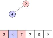
step 2: iteratively remove the maximum element, place it at the end
